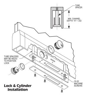
Specify either  $31/32^{\prime\prime}$  or  $1-1/8^{\prime\prime}$  cylinder height. Order 4006 strike and cylinder(s) separately if required.
